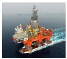
Semi-submersible rigs operate in both the midwater-, deepwater- and ultra-deepwater areas globally, depending on how the specific rig is dimensioned and equipped. Due to the good motion characteristics of Semi-submersibles, these rigs are the preferred floater type that operate in harsh environment areas. (See section 7.4 -"The Harsh Environment Segment" below).
